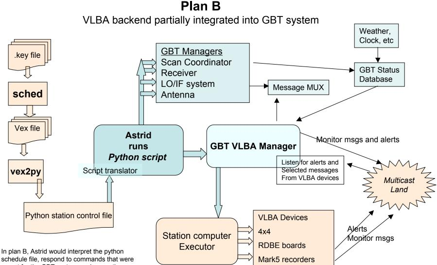
schedule file, respond to commands that were meant for the GBT system, and pass other commands to the VLBA station computer executor via the Manager, which would in turn generate commands for the backend devices.
