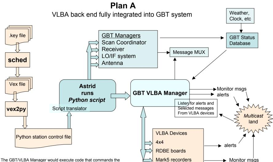
The GBT/VLBA Manager would execute code that commands the back end devices, i.e., the RDBE, Mark5, and 4x4 switch. MIB and XML commands would be sent to the device controllers directly.
