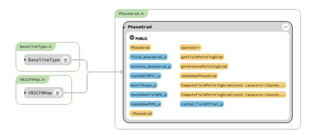
Figure 5: The members of the class VB2CFBMap and BaselineType are shown here. The public methods are shown in yellow while private fields are shown in blue. The class BaselineType is referenced as a counted pointer within VB2CFMap.
