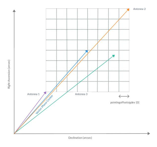
Figure 1: Shown is an illustration of the implementation. For an image with the phasecenter shown in blue, when usepointing=True the first pointingoffsetsigdev parameter decides the nearest neighbour grid size on which the antenna pointing vectors are gridded. In this case 3 unique antenna groups are found. The phase gradient is computed as the difference of the antenna pointing vector and the phase center.
