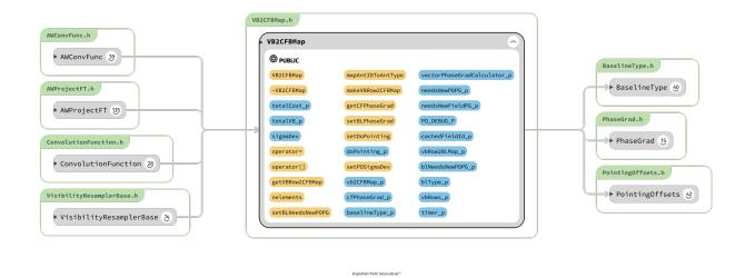
Figure 2: The members of the class VB2CFBMap are shown here. The methods are shown in yellow while fields are shown in blue. The arrows indicate the flow, Classes that are dependent on VB2CFBMap are shown to the left while the classes BaselineType PhaseGrad and PointingOffsets are referenced as counted pointers within VB2CFMap and shown leading out of it.
