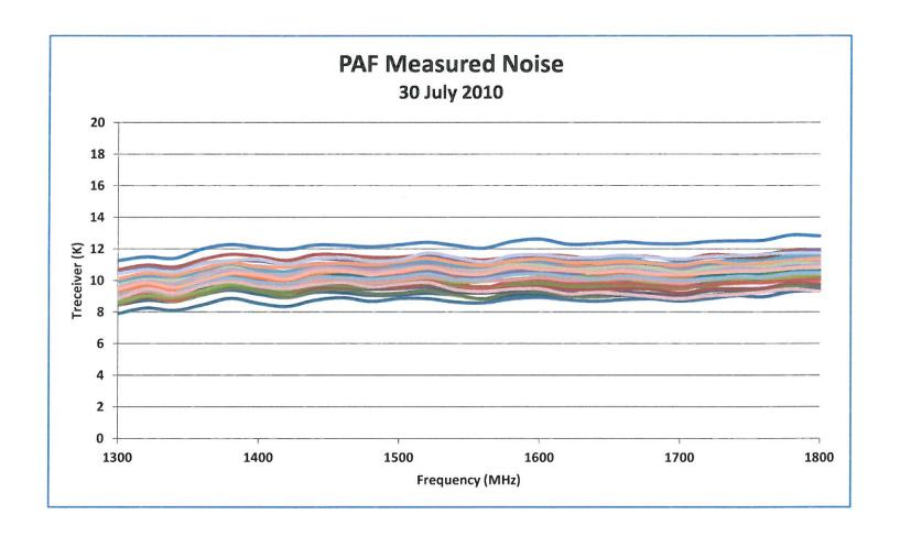
Receiver noise temperature measured using a coaxial liquid nitrogen cold load at room temperature connector.
