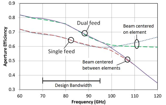
Fig. 2. Aperture efficiency of the near central beams of an 8x8 array of 6x6 mm dual feeds used to produce an f/1.9 beam. Beam centers are on an element or midway between elements. The efficiencies of an array using single TE<sub>10</sub> feeds is also shown. Above 98 GHz the sampling is less than Nyquist.
