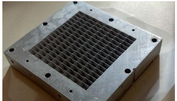
Fig. 4. Photo of the feed array with 128 apertures which are fed in pairs. The total size of the array is 48 mm square.
