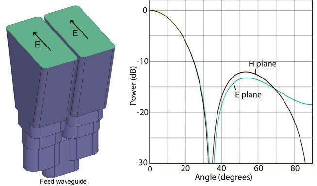
Fig. 1. Solid model of the dual feed, and E and H plane cuts through the pattern at 90 GHz. Each feed is 2.75 x 5.9 mm.
