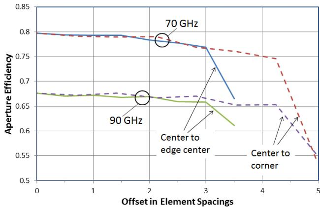
Fig. 3. Sensitivity vs beam center location in the array at 70 and 90 GHz along two lines from the array center outward. One element spacing is 0.71 HPBW at 70 GHz, and 0.92 HPBW at 90 GHz.
