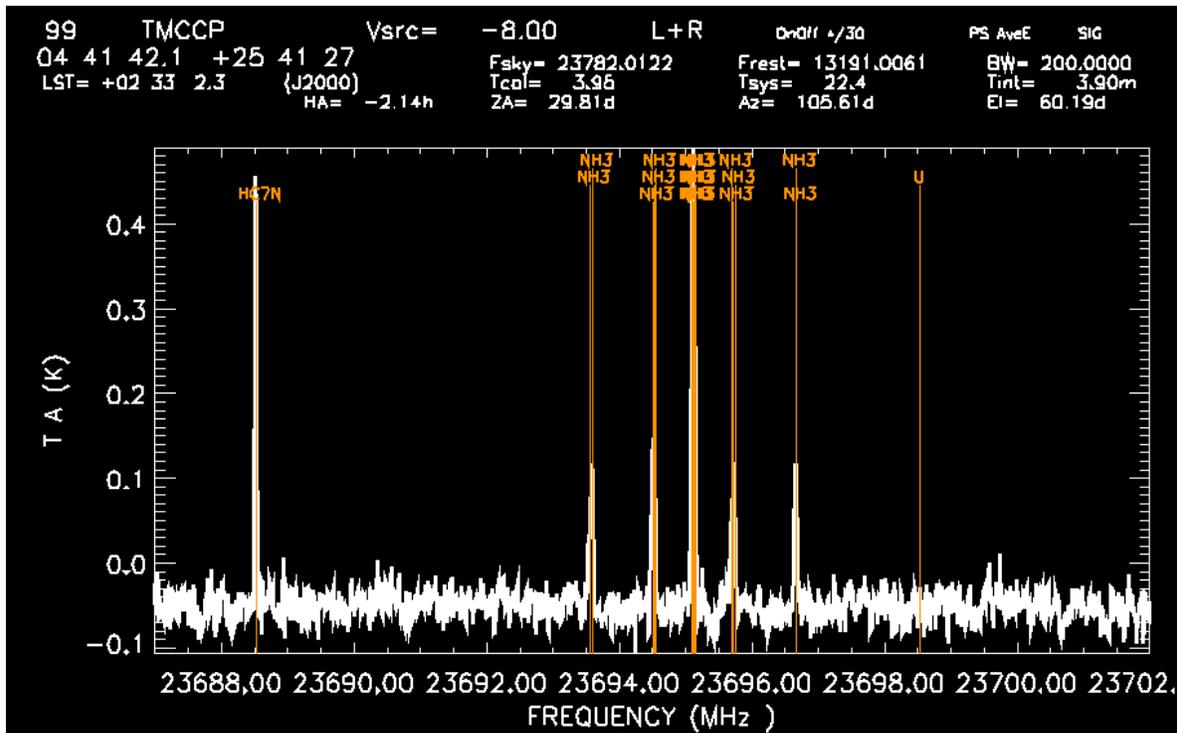
*K1 spectrum of Taurus Molecular Cloud Cyanopolyene peak. The Ammonia and HC7N lines are clearly visible in a 4 minute observation.*
