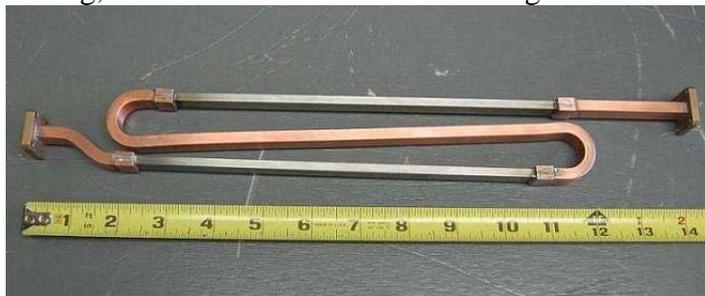
4. Integrated sliding waveguide thermal transition: Shown is the assembly used in the 1 pixel test receiver during lab tests. Each unit provides thermal isolation and flexing for the two polarizations from a single pixel. Waveguide from the cyro amps output is connected to the top. The top portion is cooled to 50K, the bottom part remains at
