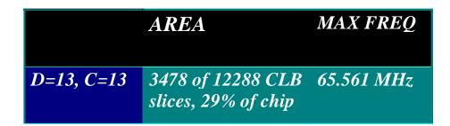
This has 16 filters, with 2 outputs each, optimized for symmetry
