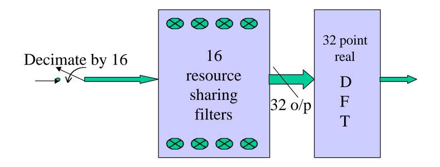
Since each filter convolves alternate samples, giving two outputs, one a convolution of even samples and the other a convolution of odd samples, it also acts to decimate by 2. So, the initial decimator needs to decimate only by 16.
