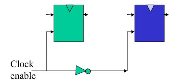
Instead of positive and negative DFFs, enable FFs can be used to convolve alternate samples. This clock enable also can be used as the select line to the muxes and demuxes.
