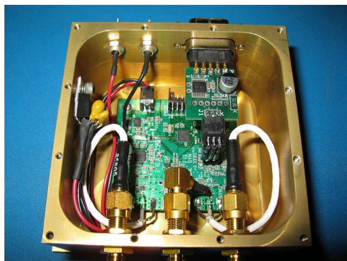
Figure 17 - Valon 5007 RFI Box Internal Wiring
