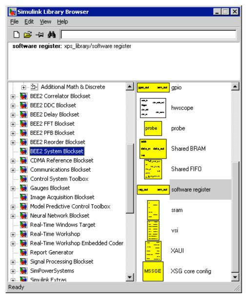
7. Add 1 instace of XSG core config and 2 instances of software register
