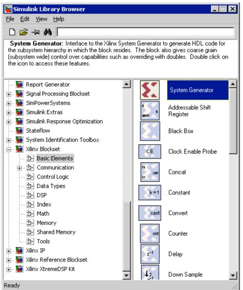
3. Add 1 instance of Counter and 1 instance of System Generator
