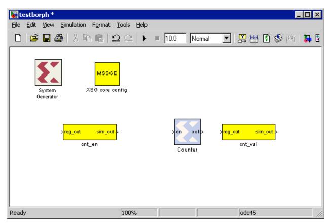
Name the instance of **sofware register** on the left of Counter as **cnt\_en**, while naming the other instance as **cnt\_val**.
