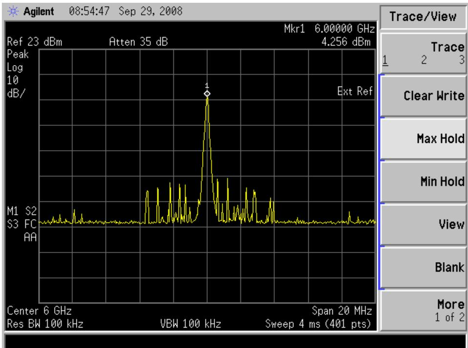
Figure 1 - monitoring receiver and source, ½ hour peak-hold
