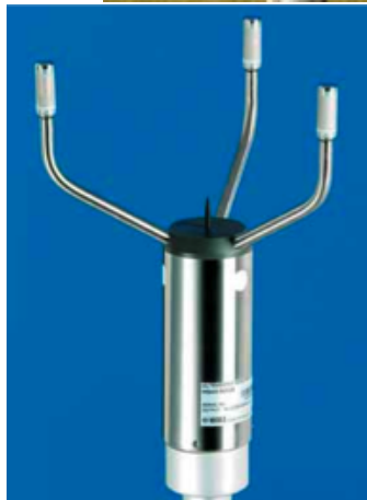
Figure 3: Clockwise from upper-left: Metek USA-1, R. M. Young 81000, Campbell Scientific CSAT3, and Vaisala WS425 sonic anemometers.
