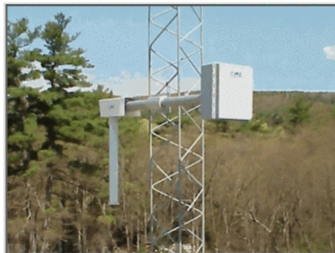
Figure 2: Yankee Environmental Systems MET-2010 Precision Meteorological Thermo-Hygrometer.
