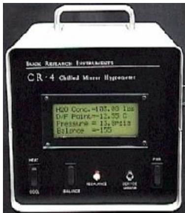
Figure 1: Buck Research CR-4 chilled-mirror hygrometer.
