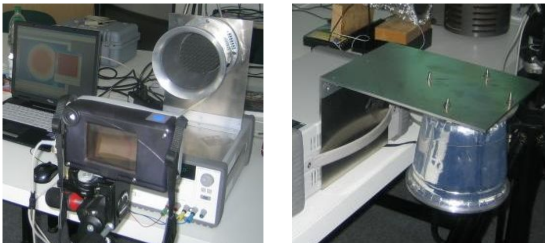
Figure 23: Horizontal (left) and vertical observing position for the IR test of the pyramidal pre-prototype target.
