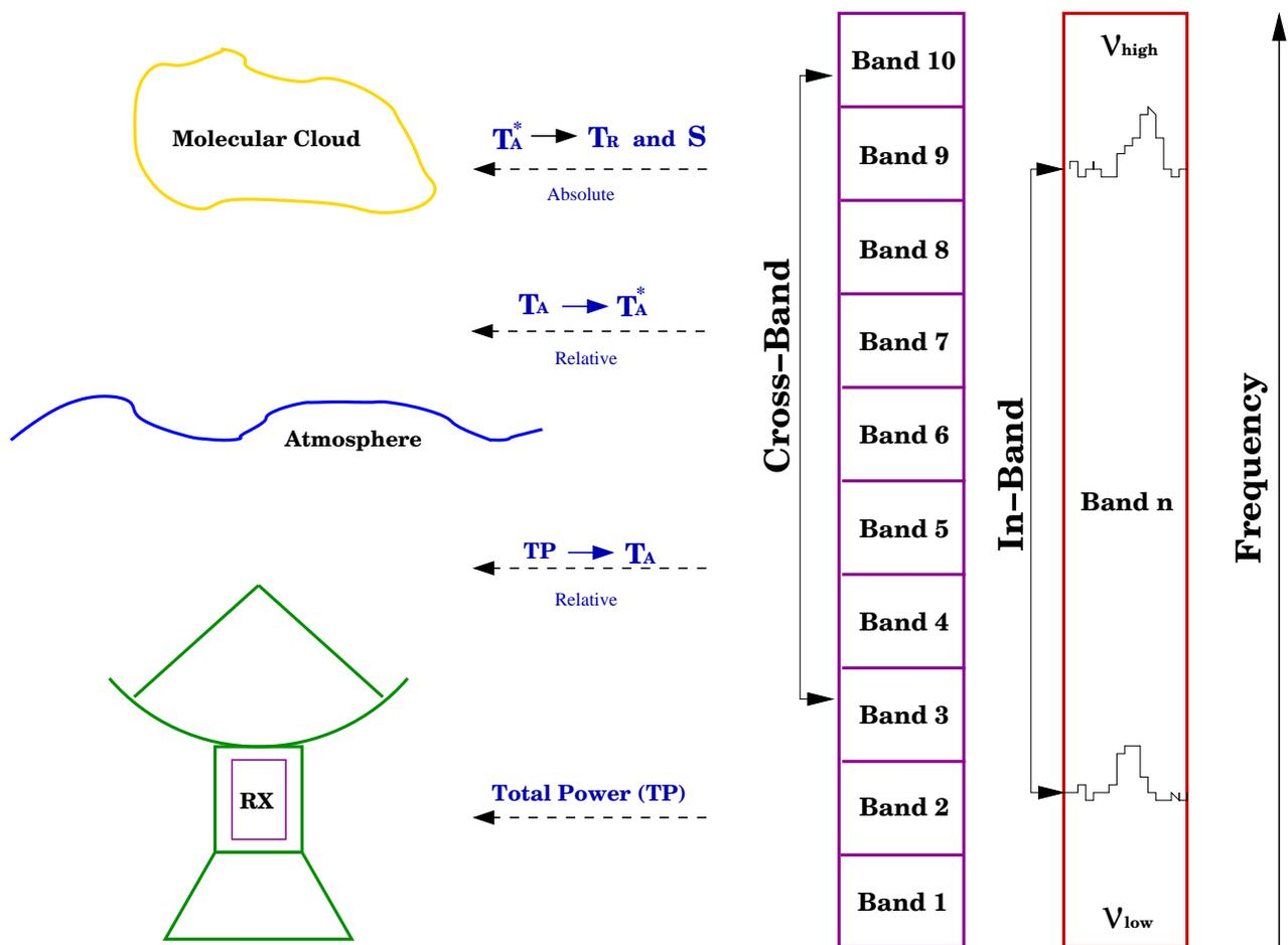
Figure 1: The amplitude calibration ladder and definition of terms. The left half of this diagram shows the steps taken to determine the absolute amplitude of a source, from total power (TP) measurement to application of a flux standard measurement ( $T_R$  and  $S$ ). The right half shows the definitions of in-band and cross-band amplitude calibration.
