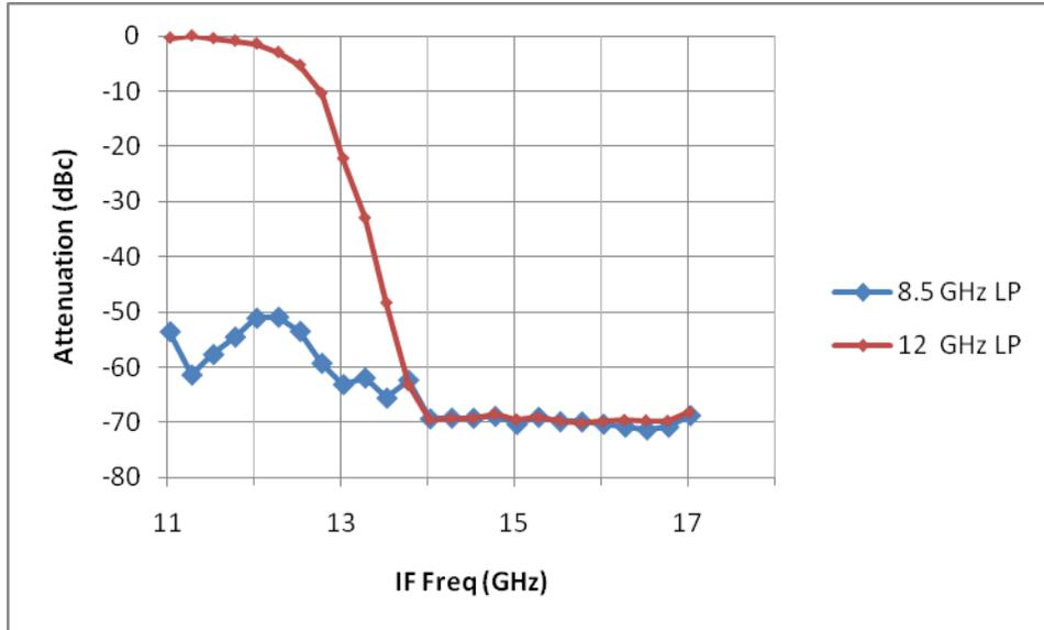
**Figure 4. End-to-end response of an IFDC for the 8.5 GHz LP filter and 12 GHz LP filter paths. Attenuation values are with respect to a signal in the desired response band.**
