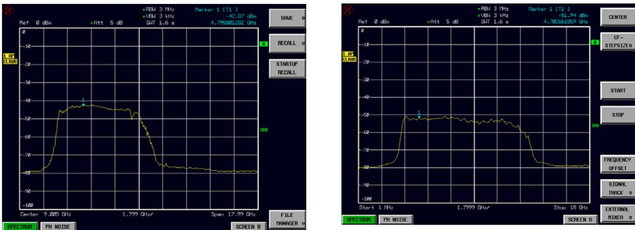
**Figure 2 Measured IF response of FE 08. Left Band 6, Right Band 9**
