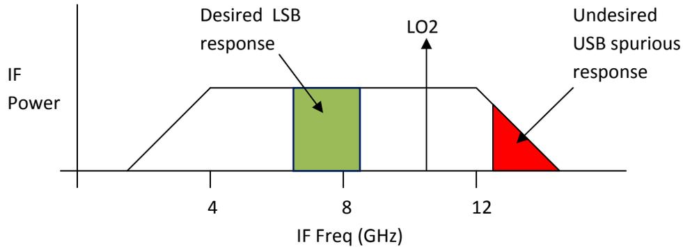
**Figure 1 Desired and undesired response with LO2=10.5 GHz**
