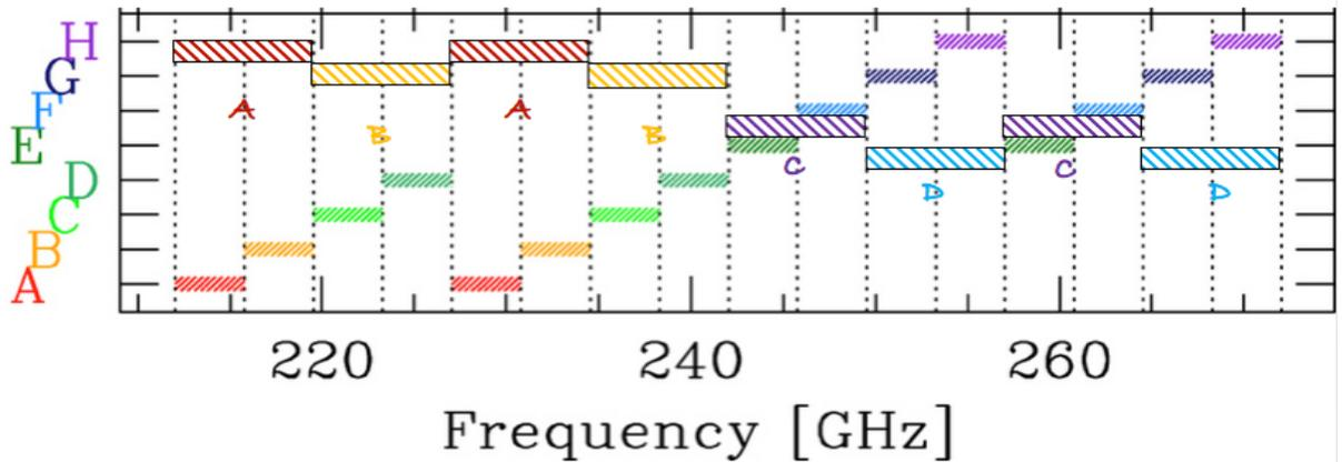
Fig. 6.— A diagram showing the eight Band 6 tunings (Lettered, left) needed to cover the frequencies of the [C II] line at redshifts of 6 to 8 in the ALMA ASPECS spectral scan of the Hubble UltraDeep Field. The eight settings needed using the upgraded correlator are shown in the upper bars, noted by script letters.
