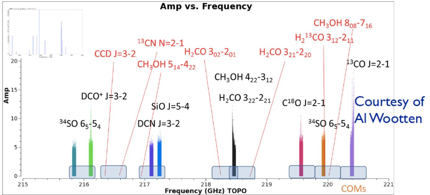
Fig. 2.— Typical protostar/protostellar disk spectral setup for ALMA using the upgraded correlator. Many more important lines (red) can be covered with the upgraded correlator capabilities.
