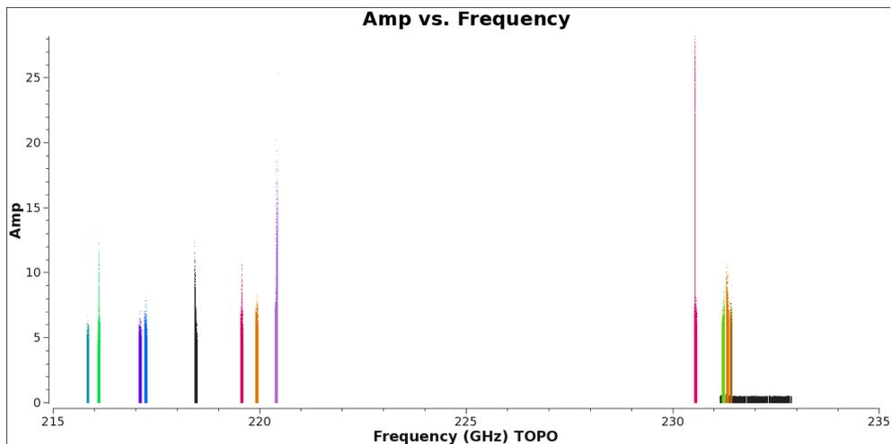
Fig. 1.— Typical protostar/protostellar disk spectral setup for ALMA. Cold gas probes the molecular envelope and disk. Modest masses limit kinematic linewidths. As a result, the science requires high resolution (a low resolution continuum window is also needed, shown in black, for calibration). The twelve high resolution windows, of bandwidth 58MHz, cover some important lines, but many important lines cannot be covered with the current correlator capabilities.
