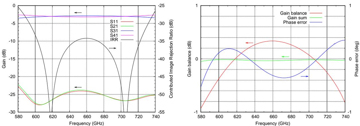
Figure 3. a (left): Representative set of S-parameters of the simulated hybrid and the hybrid's contribution to the image rejection ratio. Because of symmetry, each of the other S-parameters is identical to one of the four plotted ones. The vertical lines at 600 and 720 GHz indicate the band edges. b (right): The gain balance  $|S_{31}|^2/|S_{41}|^2$ , phase error  $\arg(S_{31}) - \arg(S_{41}) - 90^\circ$  and the total power throughput ("gain sum")  $|S_{31}|^2 + |S_{41}|^2$ .
