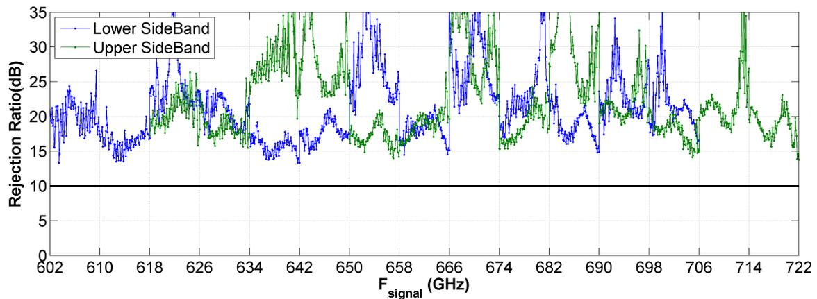
Figure 7. Preliminary measurement data of the image rejection ratio as function of RF input frequency. The ALMA specification (10 dB minimum IRR) is indicated with a horizontal line. Note that this data was obtained with an unfinished block.
