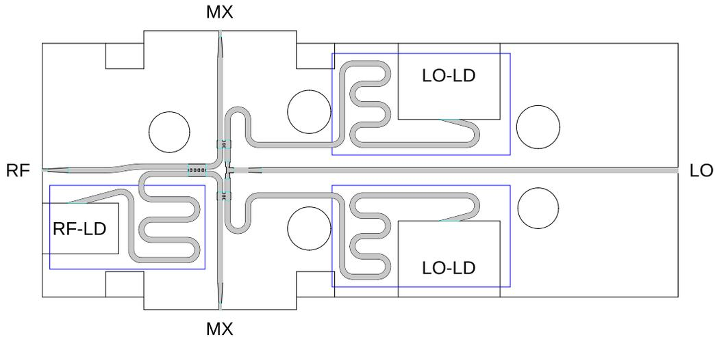
Figure 6. View on the split plane of the mixer block. RF: interface to RF feedhorn, LO: LO input, MX: interface to mixer back pieces, RF-LD: cavity for RF load material, LO-LD: cavities for LO load material. The blue rectangles indicate the areas to be coated with resistive layer.
