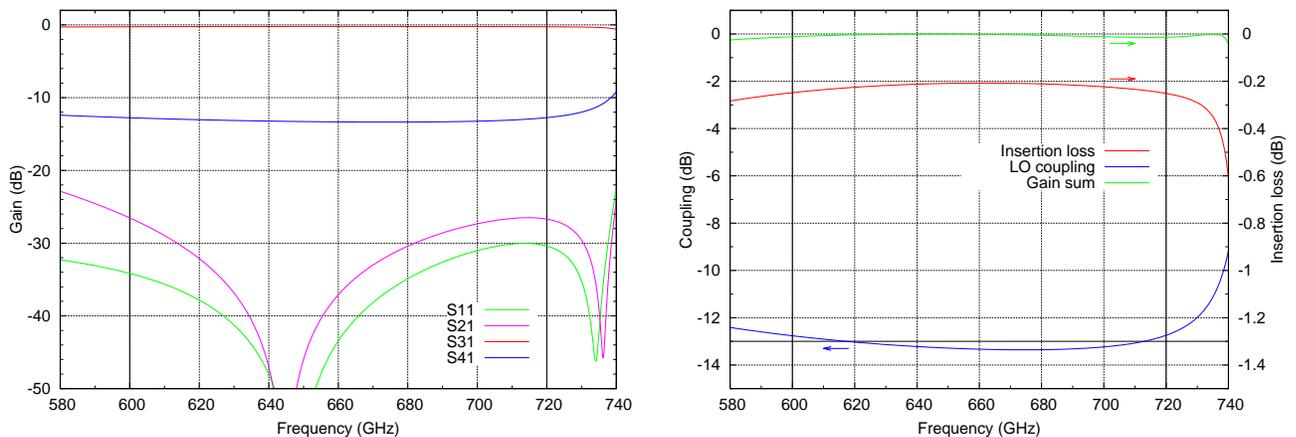
Figure 4. a (left): Representative set of S-parameters of the simulated LO coupler. b (right): Details of the LO coupling factor ( $|S_{41}|^2$ ), insertion loss ( $|S_{31}|^2$ ) and the total power throughput (“gain sum”)  $|S_{31}|^2 + |S_{41}|^2$ .
