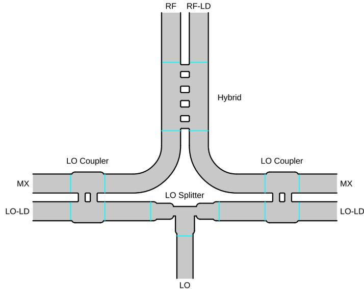
Figure 2. The central part of the waveguide structure. Port labels as follows. RF: input from feedhorn, RF-LD: RF load, LO: LO input, LO-LD: LO load, MX: mixer.
