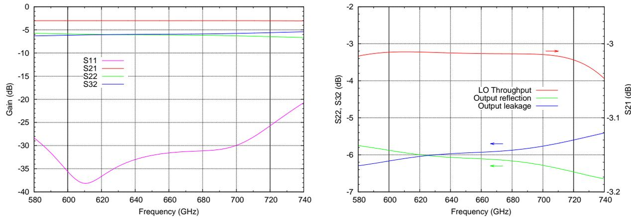
Figure 5. a (left): Representative set of S-parameters of the simulated LO splitter. b (right): Details of the LO throughput ( $|S_{21}|^2$ ), the output reflection ( $|S_{22}|^2$ ) and the output-to-output leakage ( $|S_{32}|^2$ ).
