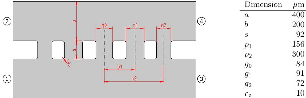
Figure 9. Dimensions of the quadrature hybrid
