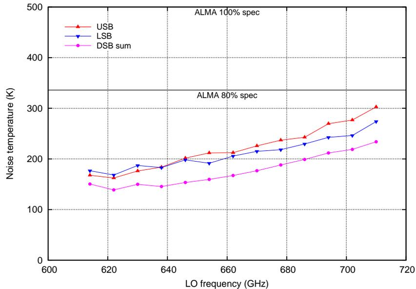
Figure 8. Preliminary noise data of both upper and lower sidebands as function of LO frequency. For reference, the sum of the DSB noise temperatures of the two individual SIS mixer devices is plotted as well. According to the ALMA Band 9 specifications, the SSB noise temperature should be below 336 K for at least 80% of the band, and below 500 K for the entire band.
