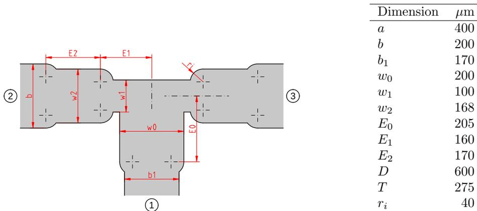
Figure 11. Dimensions of the LO splitter
