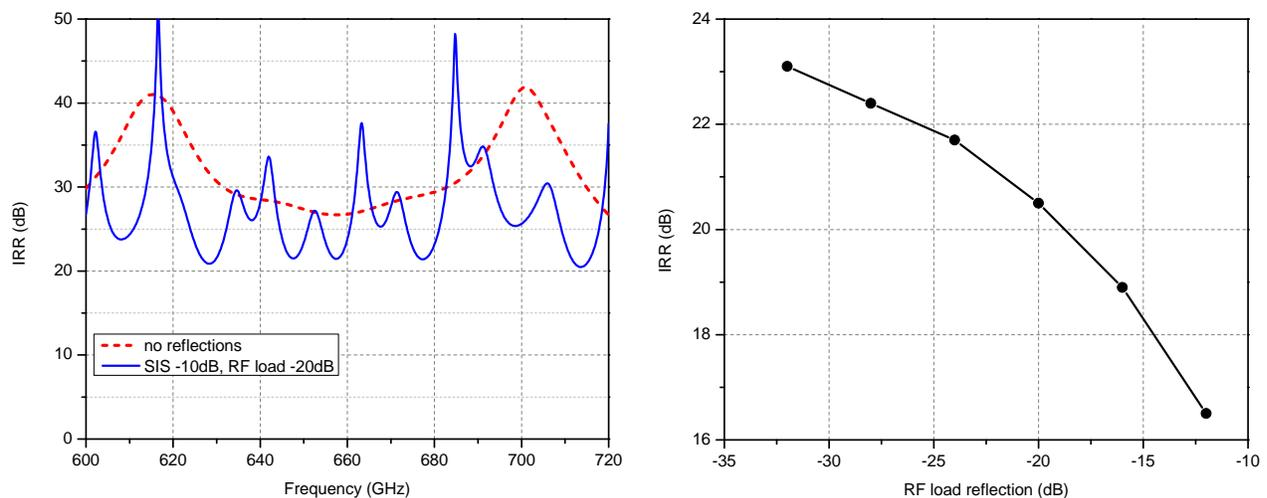
Figure 1. a (left): Simulated contribution to the image rejection ratio of the waveguide structure (*i.e.*, with ideal mixers and IF hybrid). Dotted line: no reflections from both mixers and waveguide loads. Solid line: mixer reflection -10 dB, load reflection -20 dB. Only the RF load is varied, the LO dumps are considered ideal. b (right) The minima of the IRR as determined from curves as in Fig. 1a, as function of the reflection coefficient of the RF load.
